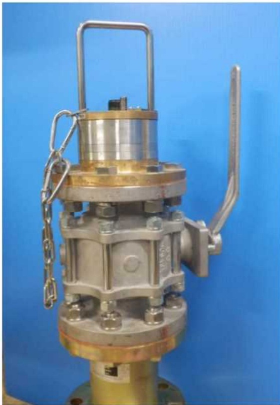
a. The Sensor is folded inside of the Valve.
