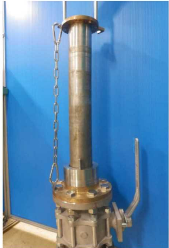
b. As the Sensor is pulled all the way up, the Chain is completely taut
