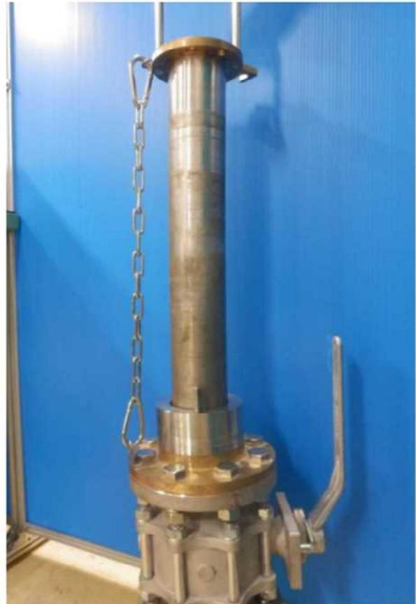
b. As the Sensor is pulled all the way up, the Chain is completely taut
